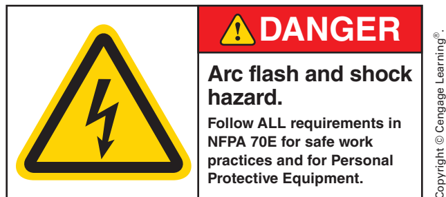
FIGURE 1-4 Typical pressure-sensitive arc flash and shock-hazard label to be affixed to electrical equipment as required by NEC 110.16 .
